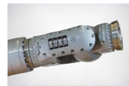
The specially sealed robot wrist with heat-resistant paintwork can withstand even the toughest conditions.
