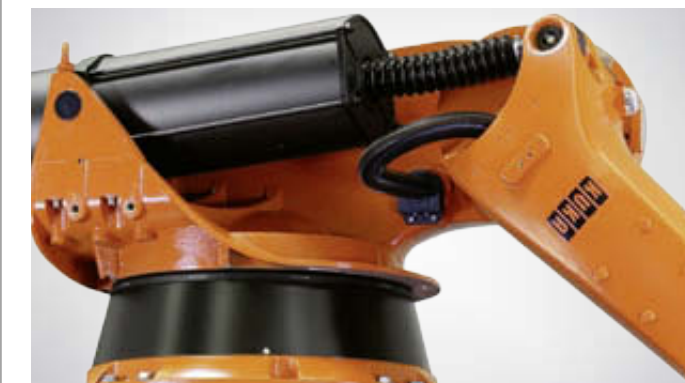
The low base is specially optimized for working downwards.
