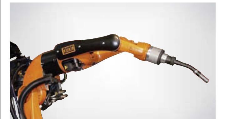
The optimally protected dress package is an integral part of the welding equipment.
