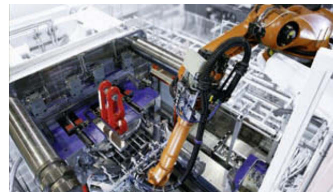
KUKA shelf-mounted robots are ideal for unloading parts from injection molding machines.
