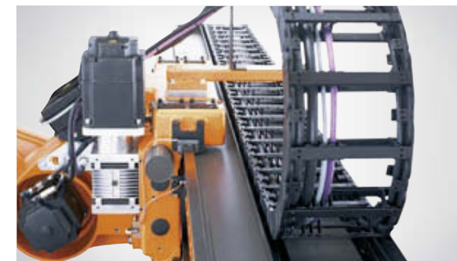
The safely routed cable carrier on the upper side of the KUKA JET, here side-mounted, allows unimpeded motion.
